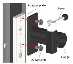
Screw the enclosed bolt into the clamp. Fasten the bolt hand-tight.
