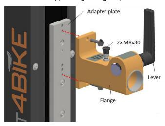
Insert the clamp into the flange:
